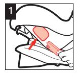
To thread the LATCH belt, put belt end with connector and adjuster through the rear-facing belt path slot.
